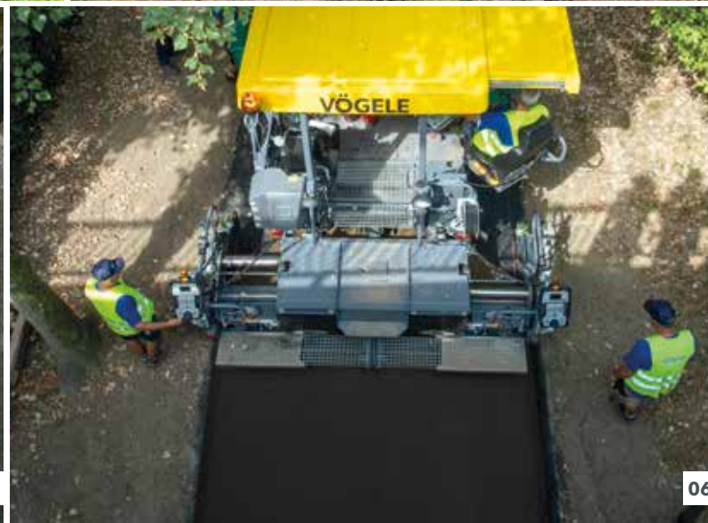
04 The paver operator's platform ensures maximum visibility. 05 Large material hopper for optimum feeding with mix. 06 AB 340 Extending Screed ensures perfect paving results.
