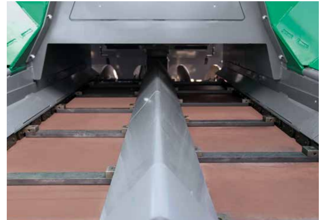
Narrow conveyor guard in the material hopper guarantees uniform material flow.
